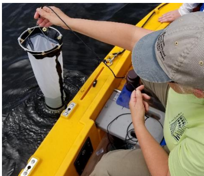
A plankton net is used to collect algae samples from the lake.
